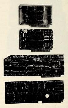
Controller cards for Apple-compatible drives (from the top): controllers from Lobo Drives; Apple Computer; the four-drive controller from Rana Systems; and Micro-Sci's controller.
