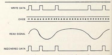
Figure 3. Data is recovered by producing a pulse for every polarity change of the read signal.
