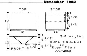
One holds 2 disk drives and the other holds the monitor. The project goes very fast. You should easily be able to complete it in one night.
