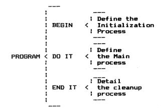
In this small example I can't really show all of the syntax used to define the Warnier' diagram method, but suffice it to say that as you work to the right, you do successively finer detail definition. The constructs "IF-THEN-ELSE", "DO-WHILE", "REPEAT" and all the rest of the classical "structured" constructs are used. At the ultimate, your program is practically complete. Perhaps this would be the subject of a good seminar. Let me hear from ye who have an interest in pursuing this subject.
