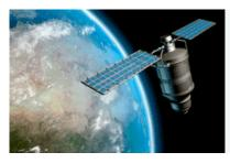
The Global Positioning System, commonly known as GPS, is a network of satellites that determines a ground based user's
