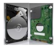
technology protects the drive mechanics and platter surfaces from shocks. WD's SecurePark<sup>TM</sup> parks the recording heads off the disk surface during spin up, spin down, and when
