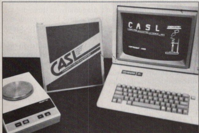
The CASL chemistry software links an Apple II computer with a Galaxy electronic balance.
