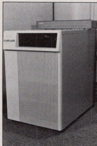
The core unit of the Cascade Speedlink local-area network for CAD systems
