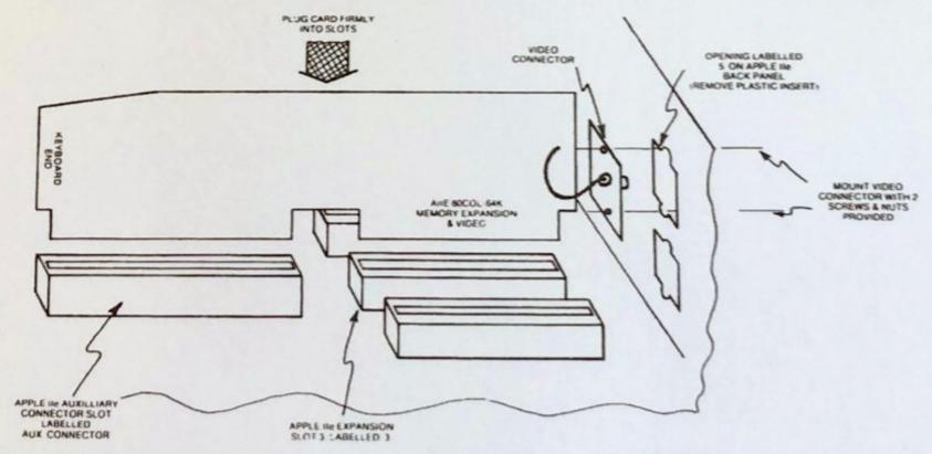
2. Hold the cable's connector against the opening. Reach behind the computer and feed the two screws through the holes above and below the opening and into the threaded holes on the connector.
