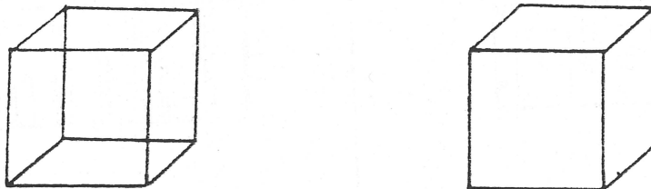
1) a wire frame object 2) hidden lines removed
