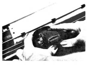
4. Hold the cartridge at an angle and slip the exposed ribbon between the printer head and the thin metal ribbon guide. It is sometimes helpful to turn the knob on the cartridge while sliding the ribbon over the print head. Gently snap the cartridge into place.
