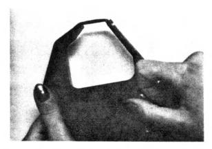
3. Take up any slack in the new ribbon by turning the knob on the cartridge in the direction of the arrow.
