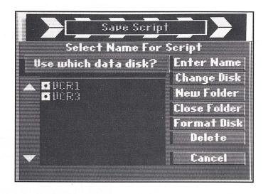
You will first be prompted to select the desired data disk from the list of available disks and disk drives that appears. When a disk has been selected, its name will appear on the first line of the file window. If there are folders on that disk, they will then be listed in the window below.
