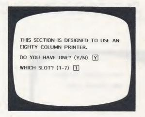
It will probably be slot 1 or 2, but if you're not sure, turn off the computer, take the cover off and check the printer card slot.
