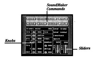
The SoundMaker program closely resembles a "sound board" used by professional recording engineers.
