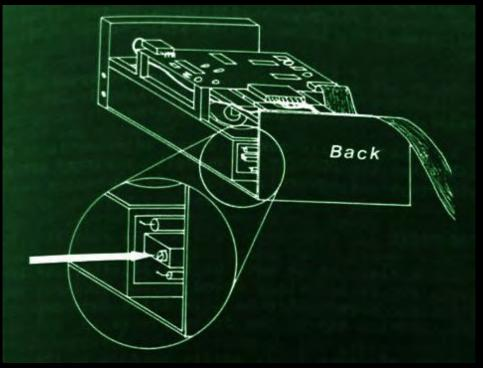
figure DISK II SPEED ADJUST SCREW
