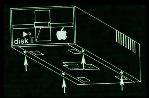
figure DISK II COVER SCREWS
