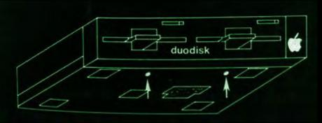
figure DUODISK SPEED ADJUST SCREW HOLES
