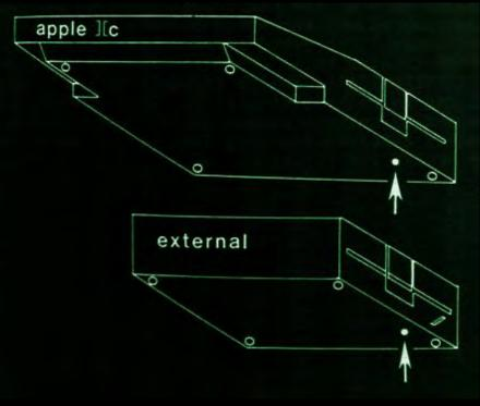
figure IIc SPEED ADJUST SCREW HOLES
