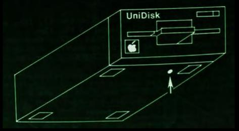
figure UNIDISK SPEED ADJUST SCREW HOLE
