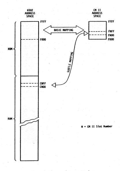
Figure 1: Diagram of Memory Mappings
