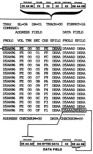
FIGURE 2.4 — ADDRESS AND DATA FIELD DISPLAY
