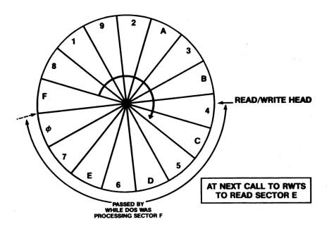
FIGURE 3.5 — STANDARD DISKETTE POSITION AFTER PROCESSING SECTOR F
