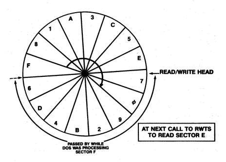
FIGURE 3.8 — 9 DESCENDING SKEW AFTER PROCESSING SECTOR F
