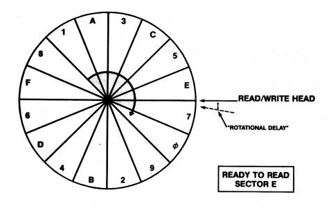
FIGURE 3.9 — 9 DESCENDING SKEW AFTER ROTATIONAL DELAY
