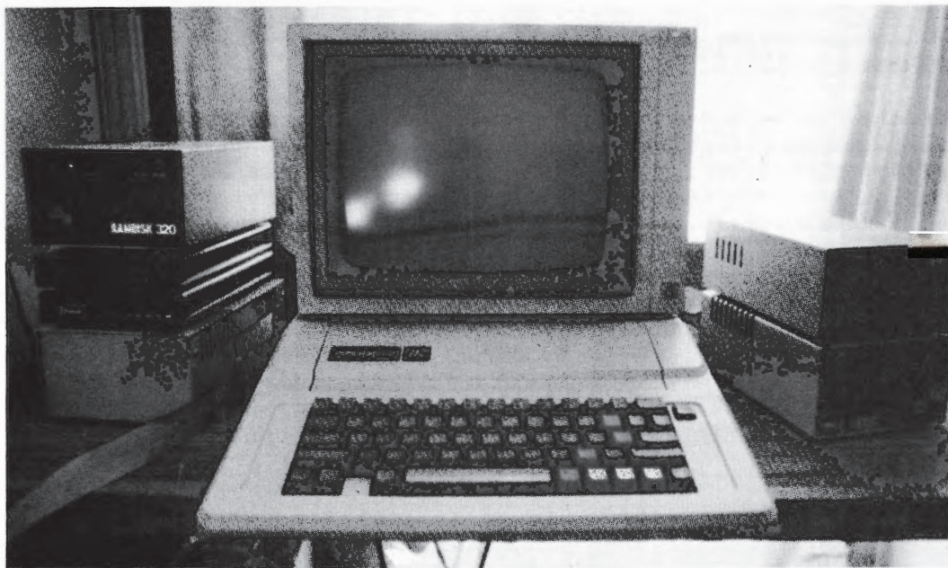
Fig. 22.6 The Axlon RAMdisk 320 to the left of the Apple is about the same size as a standard disk drive.
