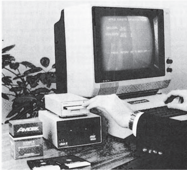
Fig. 24.7 Amdek's "Amdisk" 3 inch disk drives use a mechanism from Hitachi rather than the 3 1/2 inch Sony mechanism in the Macintosh. Unlike the Sony drives, they provide good emulation of a standard Disk II.
