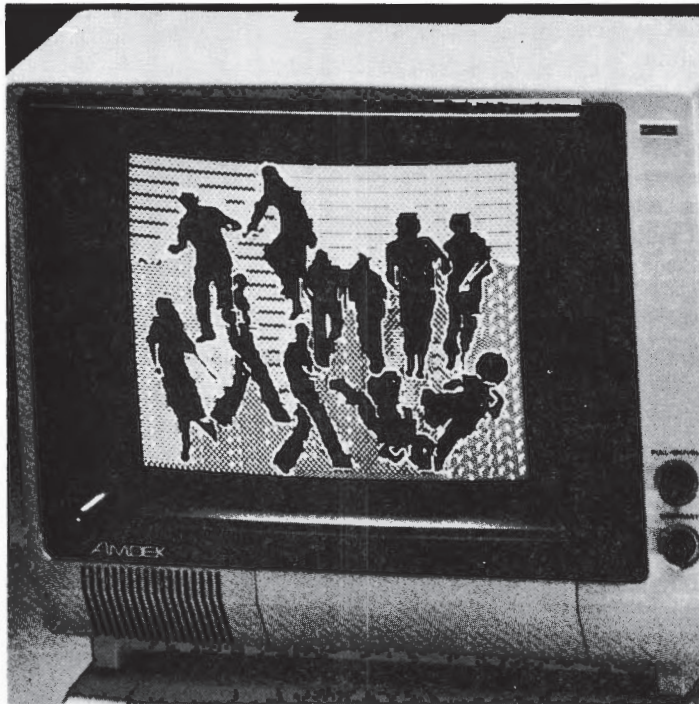
Fig. 7.5 Color I low resolution monitor with composite video input. This is an appropriate monitor for standard Apple graphics, and includes a built-in speaker to amplify sound effects.
