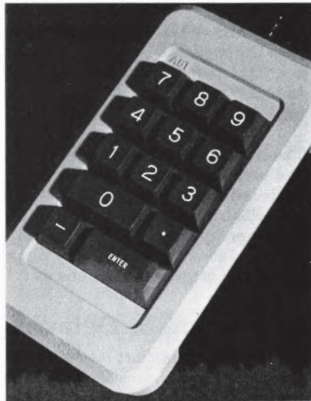
Fig. 8.7 ABT 13 key numeric pad. Separate versions are made for the II+ and for the //e.
