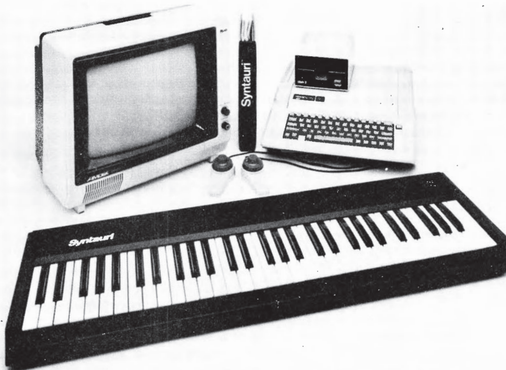
Fig. 10.5 The Syntauri synthesizer system includes the keyboard, software, and Mountain Computer instrumental music synthesizer electronics.
