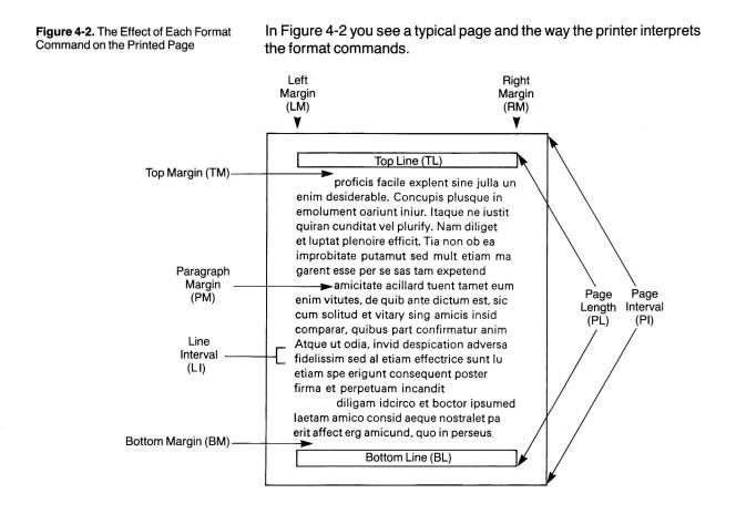
The main part of the page is the printed text, with a header (TL) and header margin (TM) at the top of the page and a footer (BL) and footer margin (BM) at the bottom.
