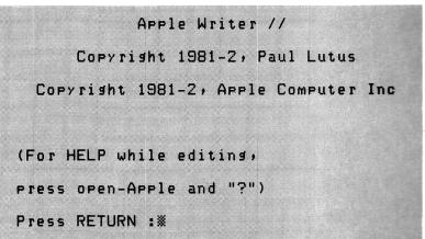
Press (RETURN) as the screen instructs. The display is blank except for a line of text at the top and a blinking white box beneath it. The blinking white box is called a *cursor*; it shows where the next character that you type will appear on the screen. The line of text is called the *Data Line*.
