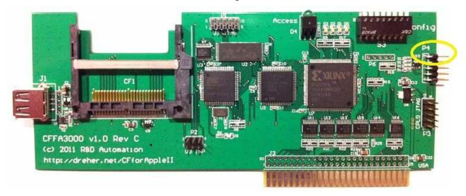
Figure 13: CFFA3000 connector to remote P4 pin 1 location
