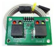
Figure 15: Remote pushbutton board.
