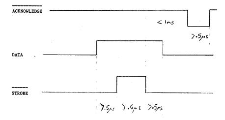
Fig 1 Interface Timing
