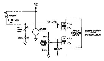
Figure 12. AD670 Temperature Transducer Interface
