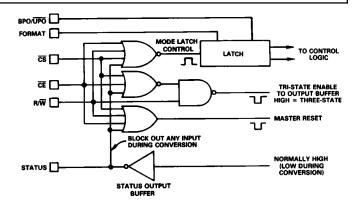
Figure 7. Control Logic Block Diagram
