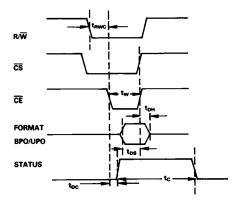
Figure 8. Write/Convert Start Timing
