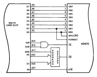
Figure 18. IBM PC Interface to AD670
