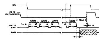
Figure 11. Stand-Alone Mode Continuous Conversion/ Single Read
