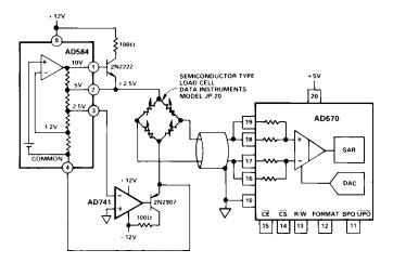
Figure 15. AD670 Load Cell Interface
