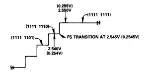
6c. Full Scale (Unipolar) Figure 6. Transfer Curves
