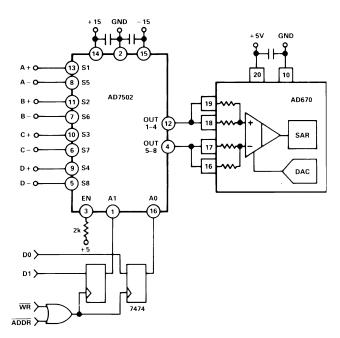
Figure 16. Multiplexed Analog Inputs to AD670
