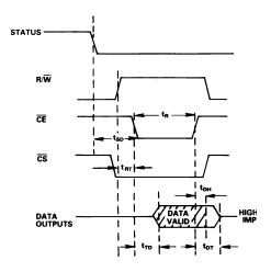
Figure 9. Read Cycle Timing
