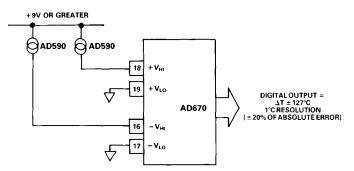
Figure 14. Differential Temperature Measurement Using the AD590
